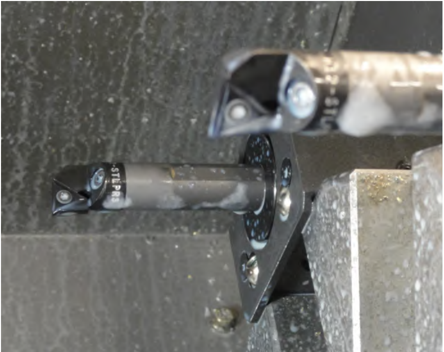
Versabar® Shanks Utilized For Multiple Machining Operations With Fast Head Change
